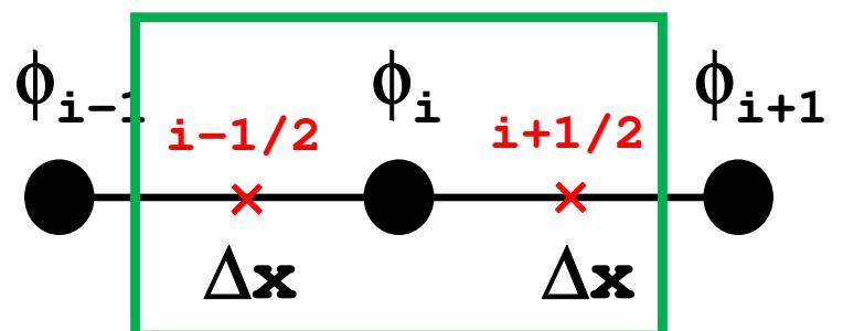
$$\left( \frac{d^2\phi}{dx^2} \right)_i \approx \frac{\left( \frac{d\phi}{dx} \right)_{i+1/2} - \left( \frac{d\phi}{dx} \right)_{i-1/2}}{\Delta x} = \frac{\frac{\phi_{i+1} - \phi_i}{\Delta x} - \frac{\phi_i - \phi_{i-1}}{\Delta x}}{\Delta x} = \frac{\phi_{i+1} - 2\phi_i + \phi_{i-1}}{\Delta x^2}$$
