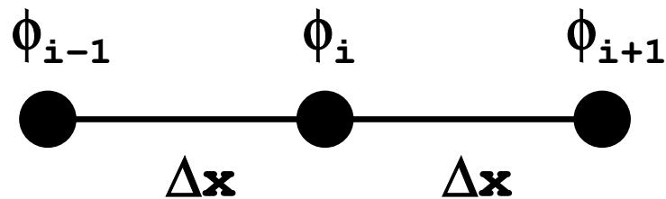
$$\phi_{i+1} = \phi_i + \Delta x \left( \frac{\partial \phi}{\partial x} \right)_i + \frac{(\Delta x)^2}{2!} \left( \frac{\partial^2 \phi}{\partial x^2} \right)_i + \frac{(\Delta x)^3}{3!} \left( \frac{\partial^3 \phi}{\partial x^3} \right)_i \dots$$
