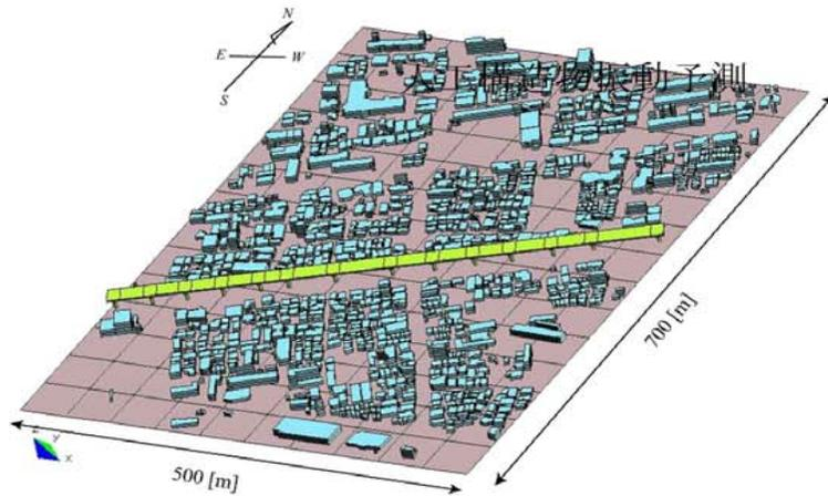
A virtual city model constructed from GIS/CAD data
